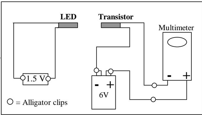
1. Connect the wires on the right (LED side) to the battery holder for the 1.5-volt. If the multimeter shows no reading or negative reading, the connections to the 1.5-volt battery holder may need to be reversed.
