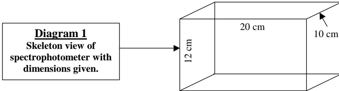
3. Two pieces of  $\frac{1}{4}$  plywood are needed for the top, one piece the same dimensions as the bottom of the box and the second piece having a length and width 1.5-cm smaller. Glue the smaller piece of wood centered on the larger piece. This will make a good, nearly light-tight seal with the sides of the case.
