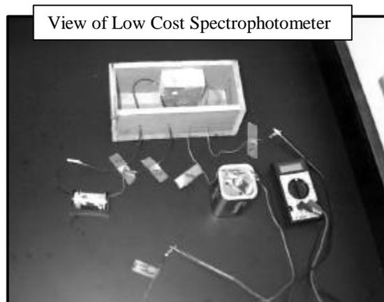
loss disconnect a wire from each battery and turn off the multimeter when finished. Check battery strength often with a battery tester to insure consistent spectrophotometer function.
